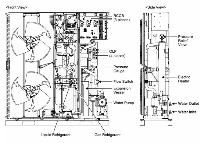
Water pump: The pump circulates the water in the water circuit.
