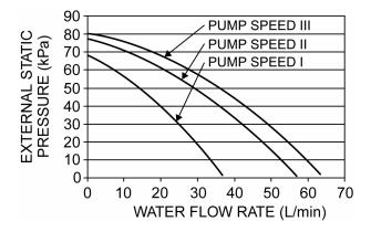
• Flow rate characteristic of mono bloc unit is as per above mentioned.
