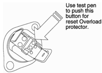
How to reset Overload protector
